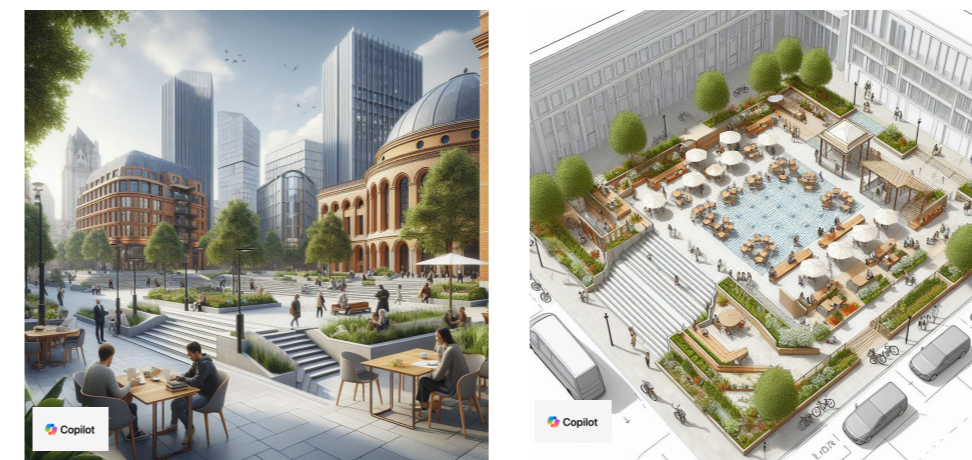
Fig 3. A street view render and axonometric plan both with features making the square not accessible and inclusive such as the varying levels and steps
