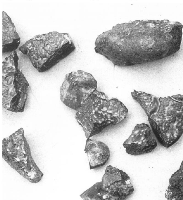
Fig. 3. Typical Chalcolithic slag (actual size) from Site 39A.
