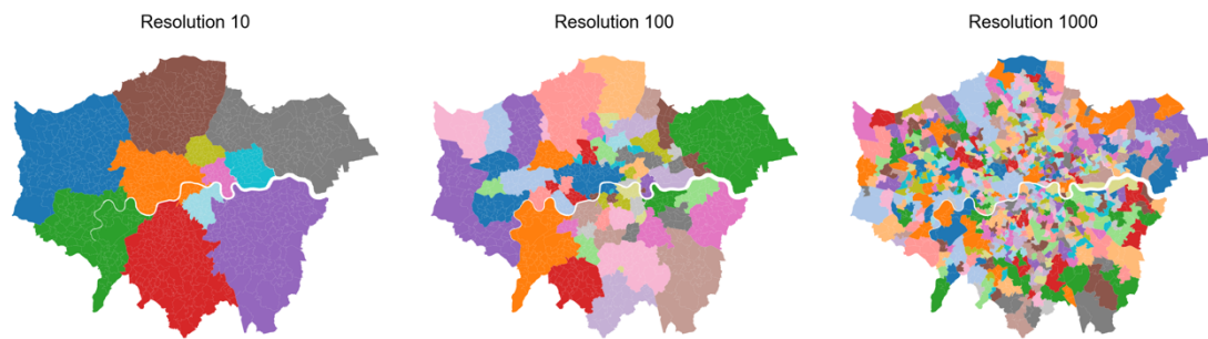
Figure 7. Modularity-based community detection was applied to O-D data of all trips, delineating urban functional zones at different spatial scales.
