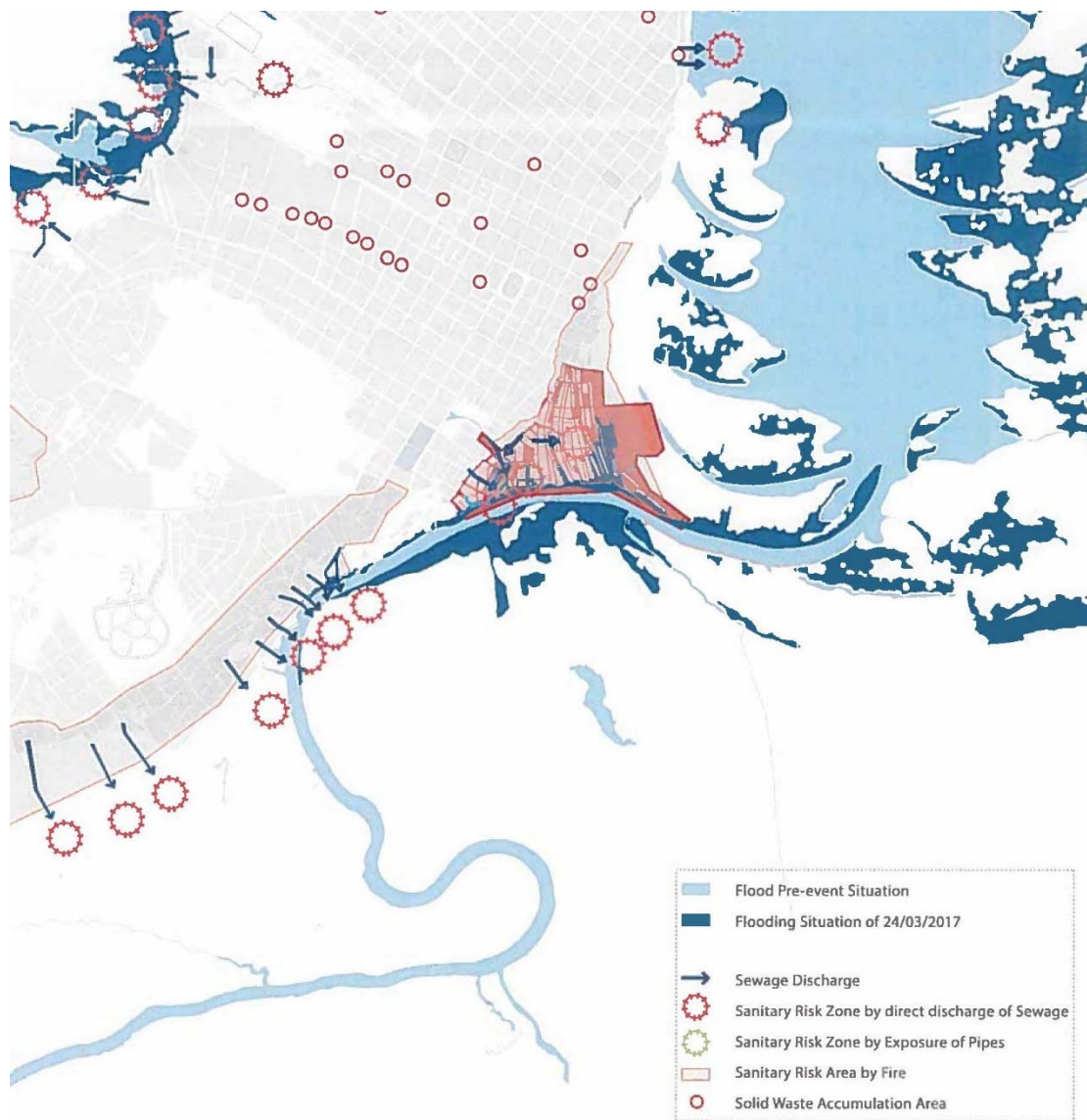
Figure. Areas subject to flooding in Iquitos. Prepared by DPU students, 2017 (multiple sources). The map clearly shows that the flooding affect more settlements than those that have been considered for relocation (in red).
