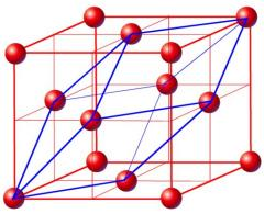
Rhombohedral primitive cell of face centred cubic system. We will work with non-primitive, conventional cubic cells.
