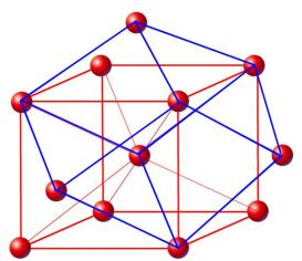
Rhombohedral primitive cell of body centred cubic system. Face centred cubic: 4 points in cubic cell (8 corner points shared 8 ways, 6 face points shared 2 ways:  $8 \times \frac{1}{8} + 6 \times \frac{1}{2} = 4$ .
