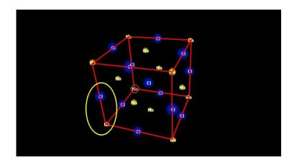
NaCl is a face-centred cubic structure. That is:
