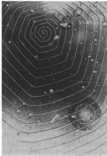
A growth spiral on a silicon carbide crystal, originating from the point of emergence of a screw dislocation (courtesy Prof. S. Amelinckx).
