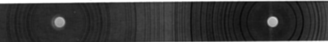
X-ray powder diffraction pattern of SiO 2 taken with CuK \alpha radiation.
