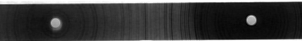
X-ray powder diffraction pattern of NaClO 3 taken with CuK \alpha radiation.
