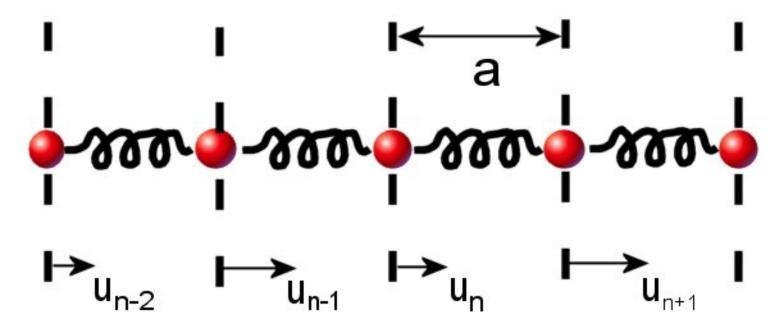
Atom n should be at a position na, but is displaced by an amount  $u_n$ . The 'unstretched string' corresponds to an interatomic spacing a. So the force on atom  $\boldsymbol{n}$  is
