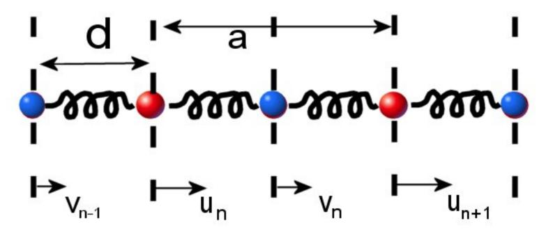
Assume atoms of mass m are at  $u_n$ , atoms of mass M at  $v_n$ . Let the atoms be d apart, with the unit cell side still a. If the force constant is
