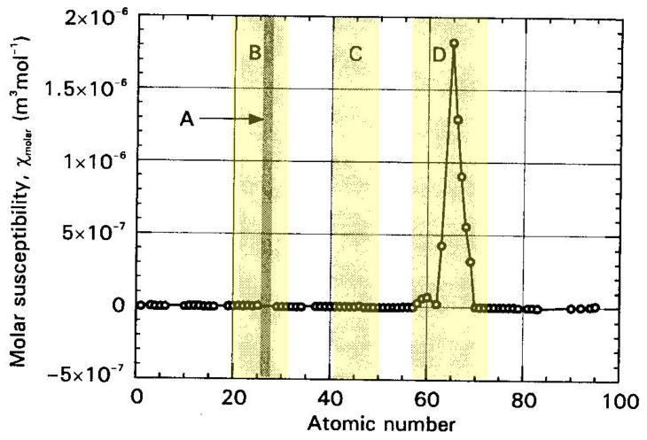
Yellow regions are ferromagnetic Fe, Co, Ni (A); first transition series (B), second transition series (C) and lanthanides (D) – all elements with part-filled inner electron shells.
