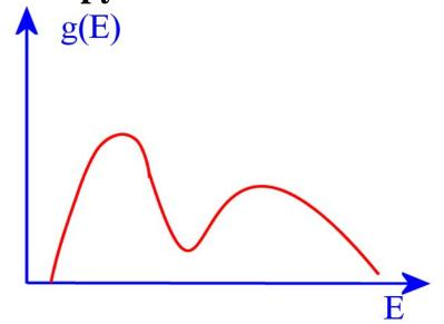
In a metal there is no gap between the occupied and unoccupied states:
