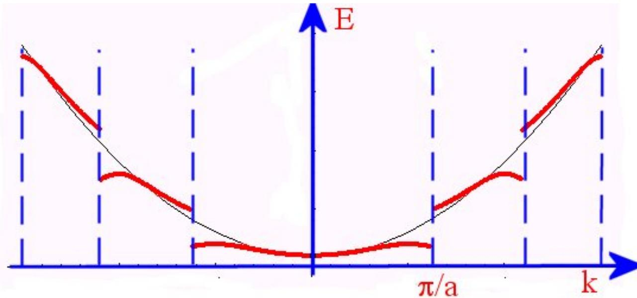
**The free electron approximation remains a good approximation well away from the edges of the Brillouin zone – only wave-vectors close to a multiple of  $\pi/a$  are mixed together and have their energies altered by the periodic potential.**
