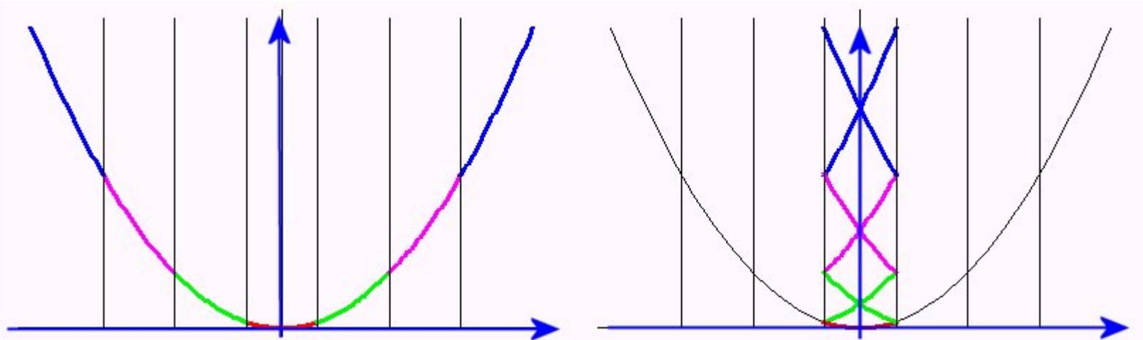
We can use the *extended zone scheme* (left) or displace all the segments of the dispersion curve back into the first Brillouin zone (right).
