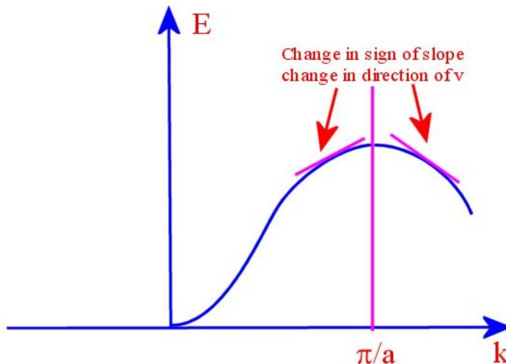
**On crossing the zone boundary, the phase velocity changes direction: the electron is reflected.**
