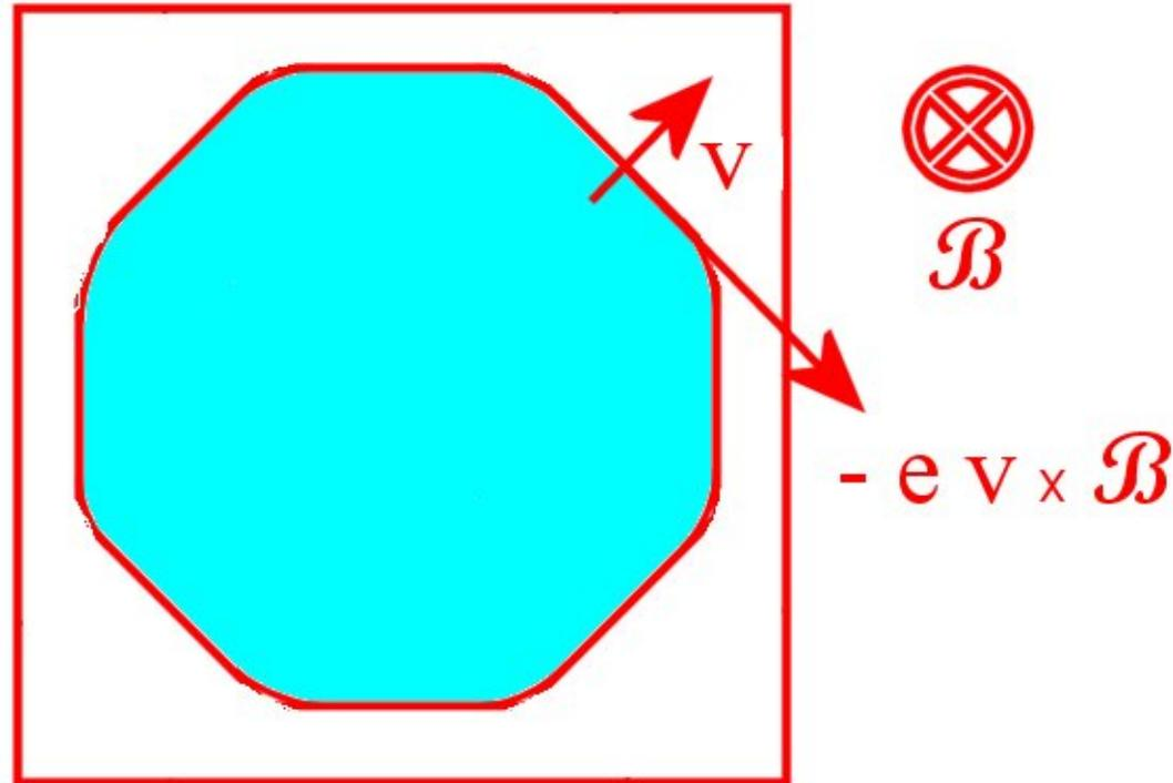
**The change in  $\mathbf{k}$  is perpendicular to both  $\mathbf{v}$  and  $\mathcal{B}$  – the electron stays on the constant energy surface.**
