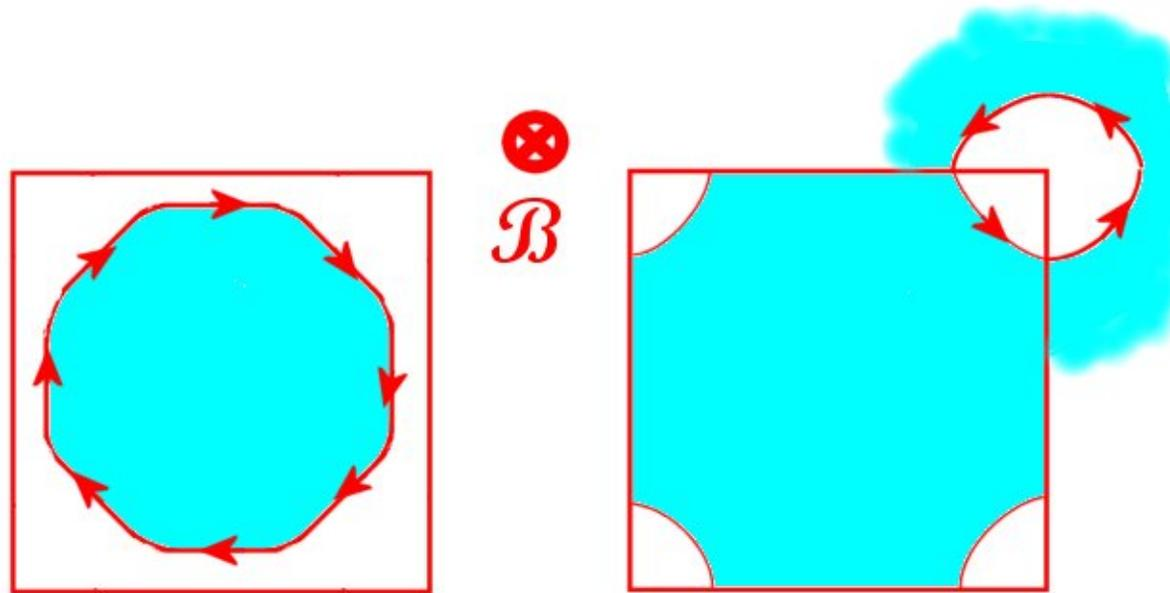
**The electrons orbit, in  $k$ -space, the opposite way round occupied or unoccupied states. The behaviour looks like that of an oppositely charged particle – a *hole*.**
