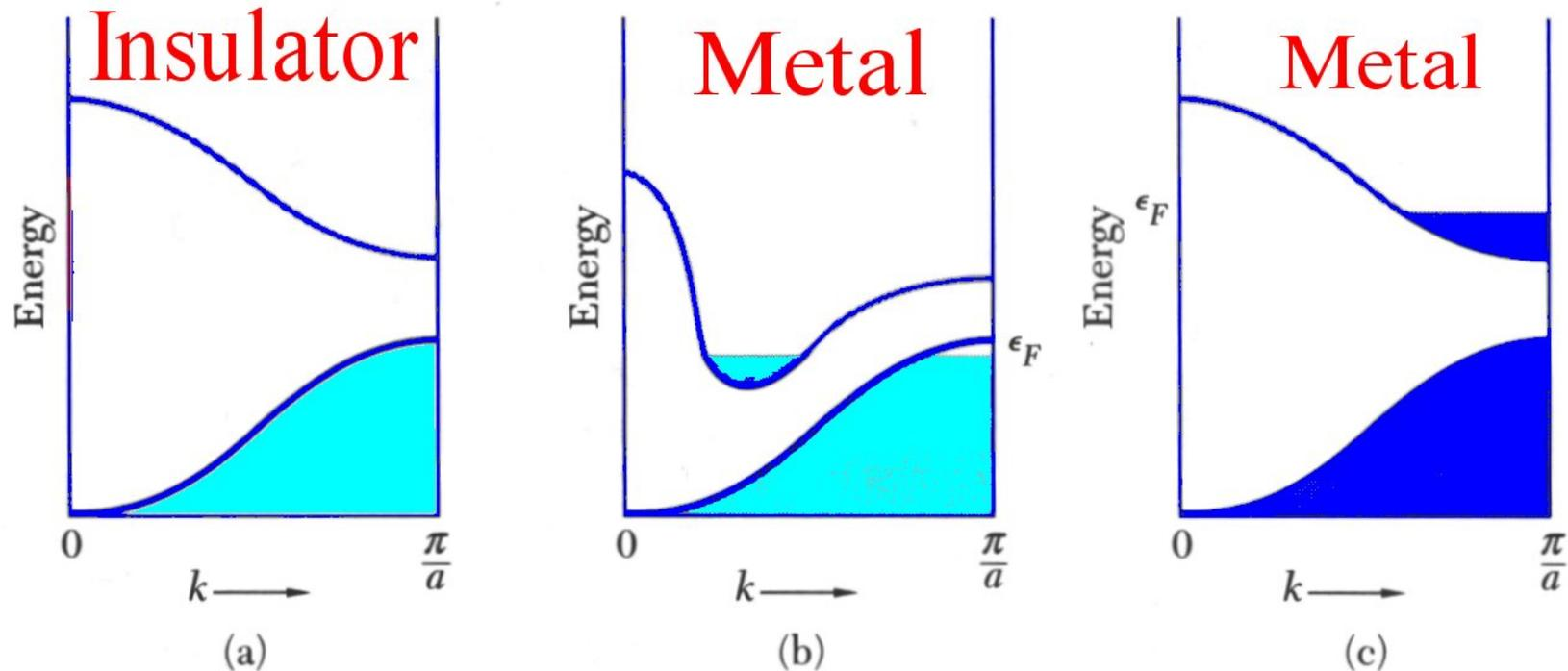
In the insulator, there is an energy gap between the occupied and unoccupied states. For a metal, there may be overlap (b) or not (c).
