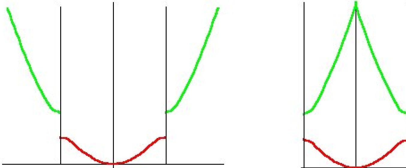
**in either the extended zone scheme (left) or the reduced zone scheme (right). Note that states further from the origin in the extended zone scheme can also be represented as higher bands in the reduced zone scheme.**
