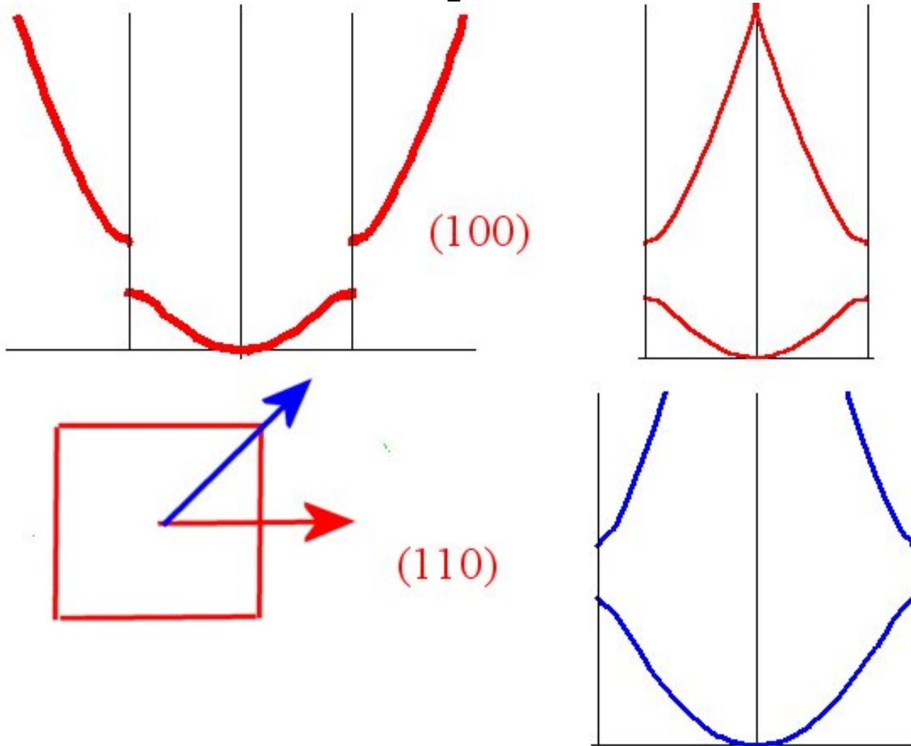
Consider a divalent metal in two dimensions. The area of  $k$ -space needed to accommodate all the electrons is equal to the area of the first Brillouin zone. We can see that the red states in the second band will start to be filled.
