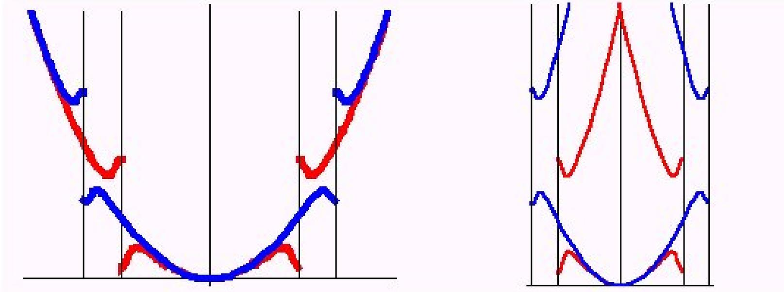
For a large gap, the whole of the first zone will be filled. This gives an insulator because if we apply a field to increase an electron's  $k$  vector, electrons at the zone boundary will be Bragg reflected back to the other side of the zone – there will be no net drift velocity. We only get current if we can excite some electrons into a higher energy band.
