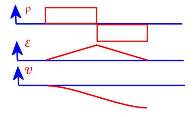
Here is the relationship between the potential through the junction and the band structure.
