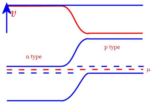
In equilibrium, we can assume there are practically no electrons on the p-type side. On the n-type side the fraction of the electrons with enough energy to move to the p-type side will vary as  $\exp(-E_{\rm g}/k_{\rm B}T)$  (those with energy  $E_{\rm g}$  above the bottom of the conduction band.)
