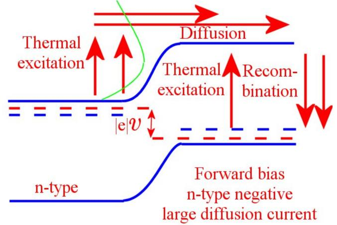
But forward bias the junction, raising the energy of the electrons in the n-type region by eV, and the number passing from n to p is increased by a factor  $\exp(eV/k_{\rm B}T)$ . Under reverse bias, the number of electrons flowing from n to p is reduced, and as there are hardly any electrons in the p-type the reverse current is very low.
