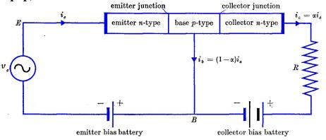
The signal voltage  $V_s$  added to the emitter voltage alters the current through the collector, giving an amplified voltage across the load resistance R.
