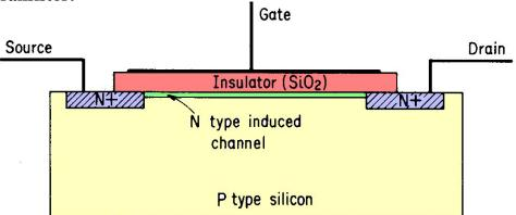
Altering the gate voltage alters the number of electrons in the induced inversion layer: current can flow between the heavily n-type doped regions.
