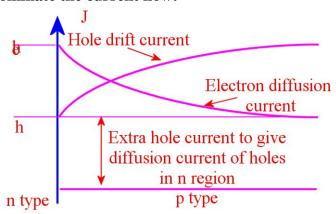
Typical diffusion length,  $l_{\rm e}$  or  $l_{\rm h}$ , is about  $1~{\rm mm}$ , much larger than the width of the depletion zone (about  $1~\mu{\rm m}$ .
