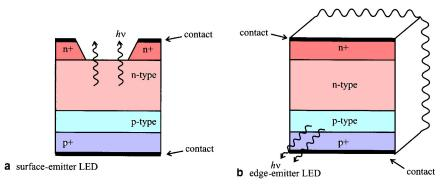
Given a population inversion (large populations of electrons in the conduction band and holes in the valence band) we can get lasing action. This can be achieved with degenerate doping –  $E-\mu$  comparable with or less than  $k_{\rm B}T$ . Also need to set structure up in resonance - multiple reflections in wave-guide structure.
