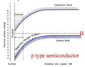
That is, with a voltage we can induce a density of *free electrons* in p-type material – called an *inversion region* – band bending effects from Poisson's equation as before.
