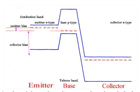
Any change in base-emitter voltage causes a large change in the electron current injected into the base. Most of these electrons flow on into the collector.
