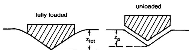
Fig. 1. An illustration of the problems introduced by the elastic sinking-in of an indentation impression under load.
