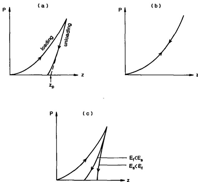
Fig. 2. Typical loading and unloading curves for (a) an elastoplastic material, (b) an elastic material, and (c) an elastoplastic coated substrate.
