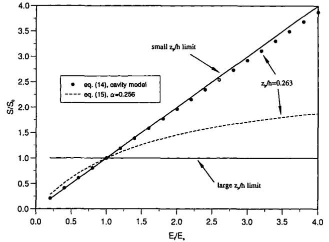
Fig. 3. Comparison of elastic unloading slopes according to the coated cavity model (eqn. (14)) and calculations by King [6] (represented by eqn. (15)), for a range of ratios  $E_f/E_s$  and various  $z_p/h$  values, for  $\nu_s = \nu_f = 0.3$ .  $S_0$  is the slope in the absence of a film.
