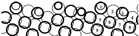
FIG. 7. Side view of refined O/Cu(104) surface structure. Bolder atoms are in the y=0 plane, while the lighter atoms are in the y=\frac{1}{2} plane. O atoms have a smaller diameter than the Cu atoms.
